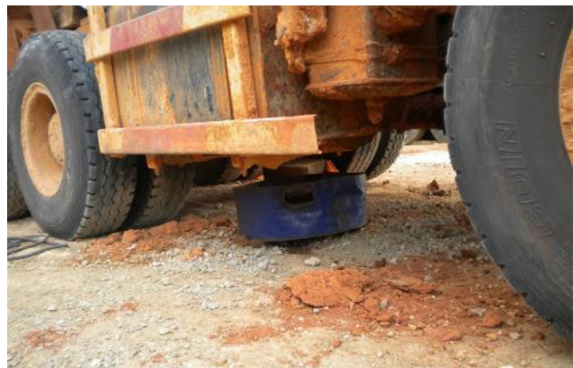
Figure 31. Use of Drip Pan During Vehicle Maintenance
