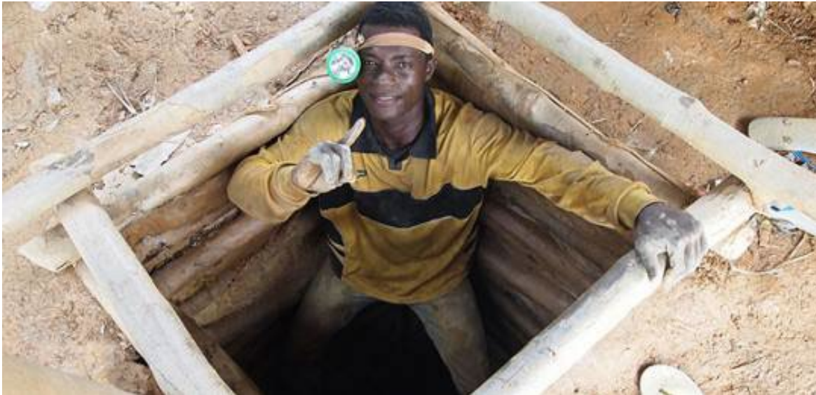
FIGURE 9. A GHANAIAN MINER AT THE OPENING OF A 15-M MINE SHAFT REINFORCED WITH WOOD. 75
