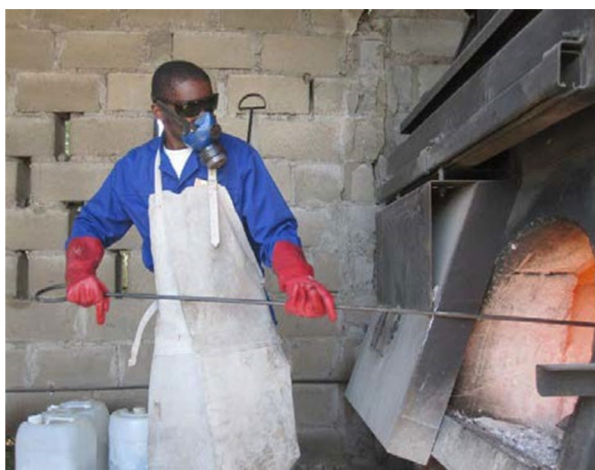
Proper PPE is crucial for individuals handling waste and operating incinerators to reduce the associated risks, including physical injury or the inhalation of exhaust. Photo Credit: Scott Ackerson
